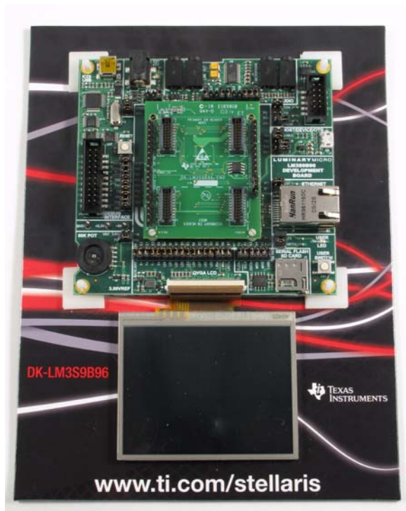
Stellaris® EM2 Expansion Board Attached to DK-LM3S9B96 Development Board (sold separately)
